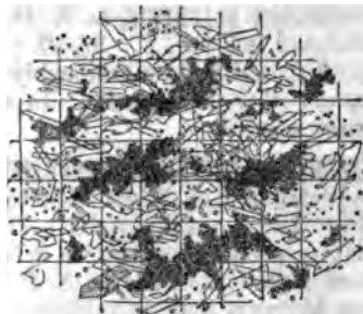
Microscopic appearance of commercial (i. e. impure) precipitated sulphur, showing the crystals of sulphate of lime (selenite).
